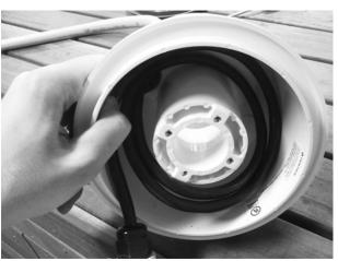
11. Pull the power cable through, leaving about 1m of cable to allow inspection of light above water surface.
