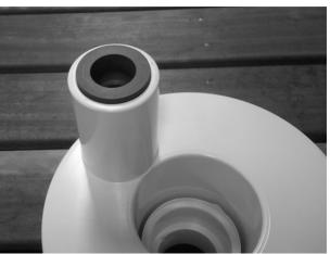
2. Insert the glued conduit adaptor into the glued socket on the niche. Allow time for glue to set (refer to gluing instructions from glue manufacturer).
