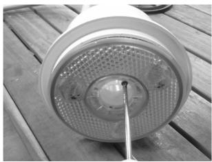
12. Push in LED light and fix with 4 screws provided.
